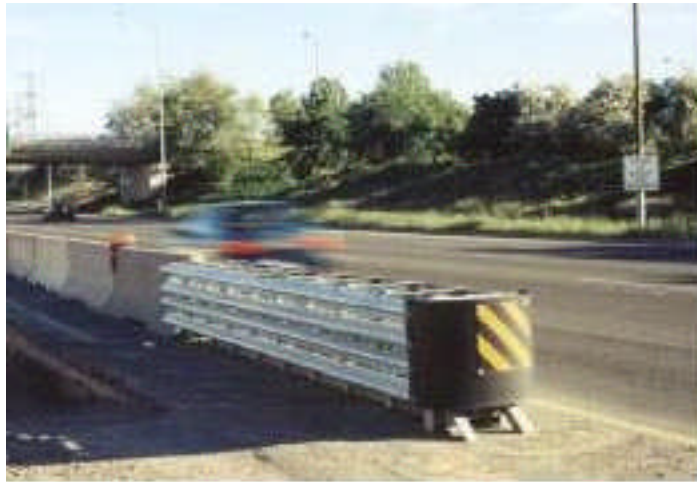
A TRACC installed in a Toronto, Canada Construction Zone
