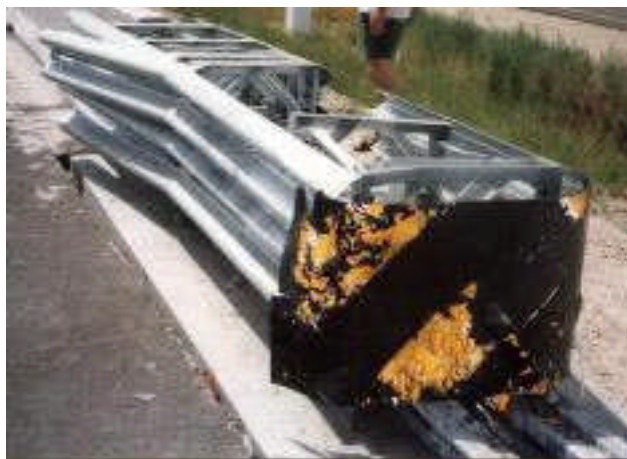
Damaged TRACC in Boise, Idaho
